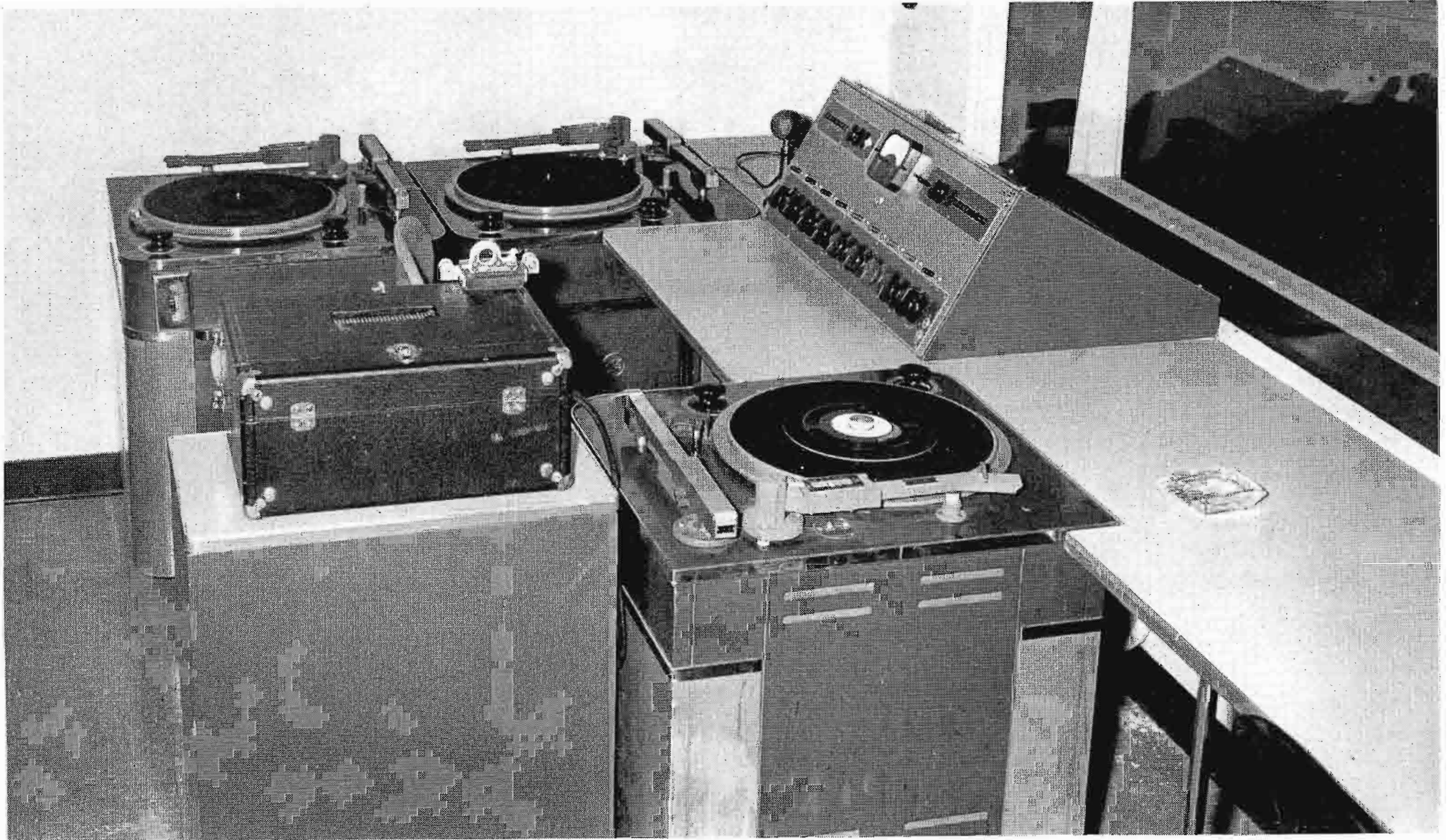
FIG. 8. Availability of a third turntable in each control room is responsible for much of the smoothness of WMCA operations. Control room for Studio "A" with three Type 70-D turntables is shown.
