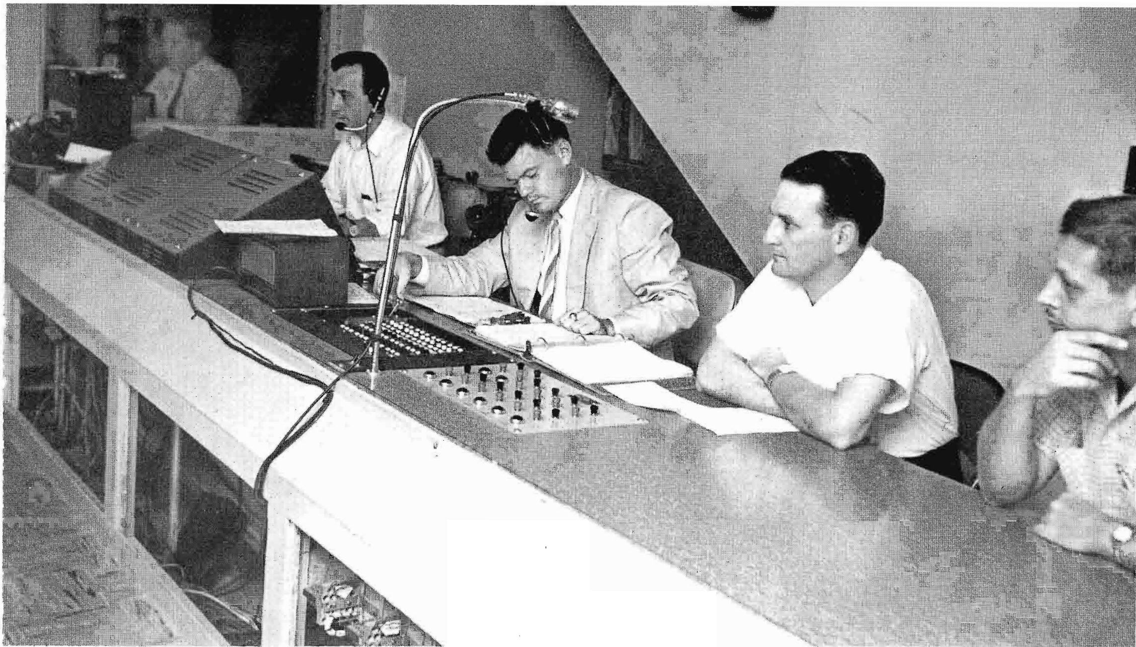
FIG. 10. Studio "A" production control room, larger of two control rooms. Elevated three feet to effect good visibility. Twenty-foot control desk extends full width of room. Equipment looking from foreground consists of: lighting remote control, intercom control, TS-20A Video switcher, TG-15A special effects, BCM-1A mixer, BC-2B consolette, tape recorder and play back.
