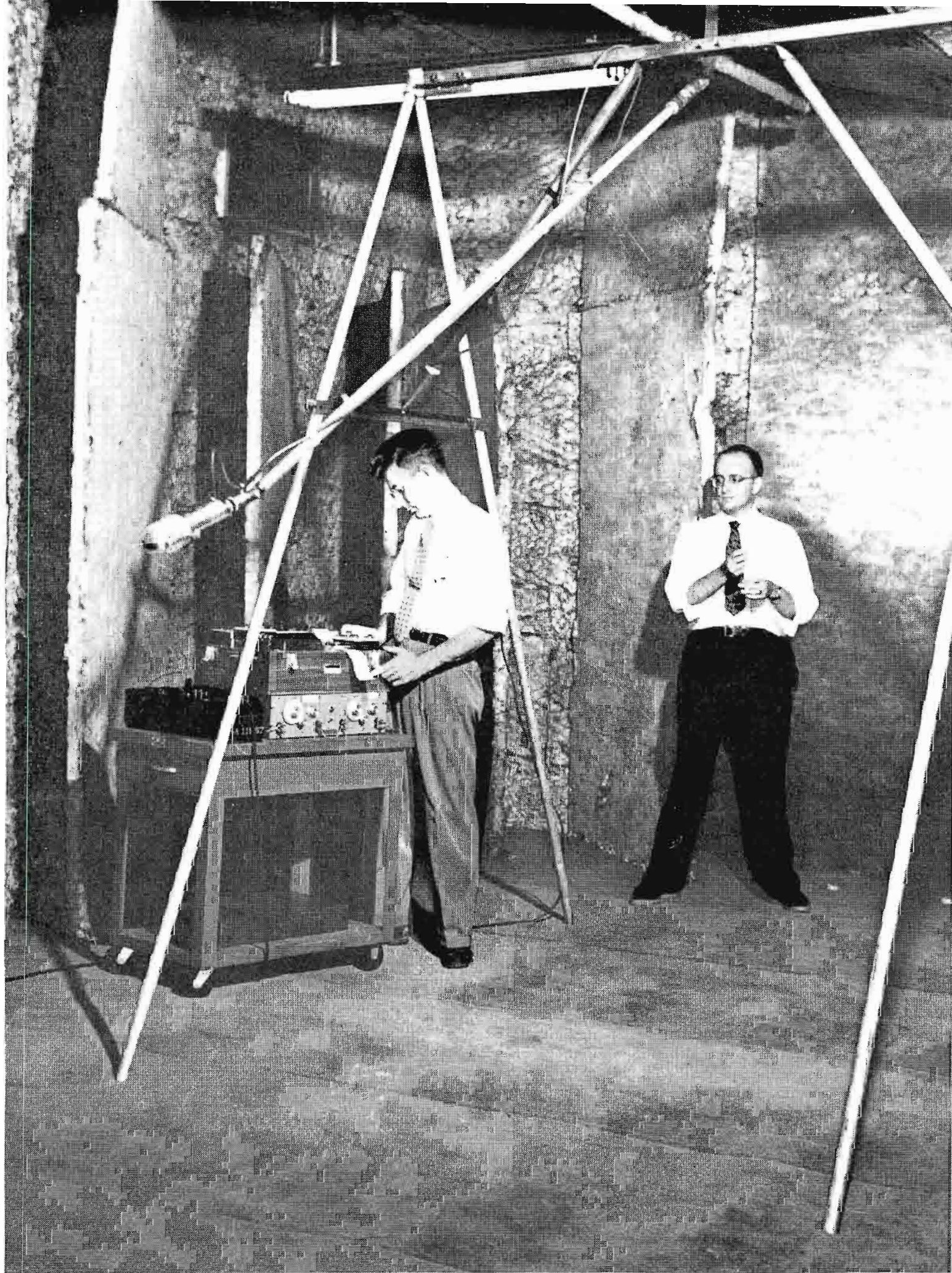
FIG. 1. Anechoic, or echoless room used for testing microphones at RCA. Wedges of Fiberglas 3 to 6 ft deep line the room.
