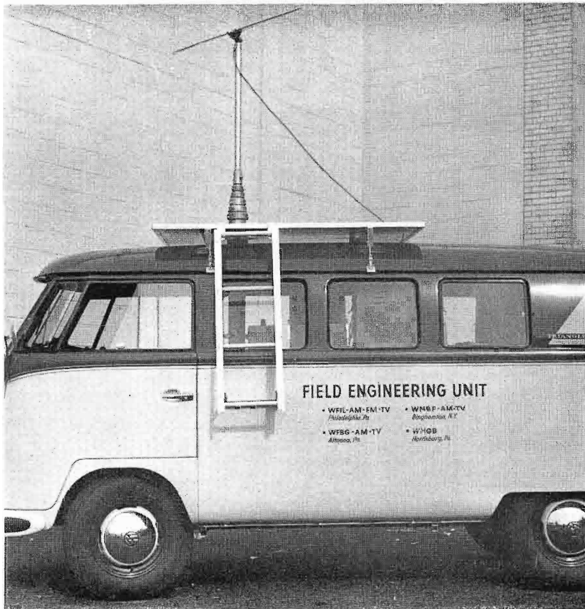
FIG. 6. View of bus showing rigid metal platform for supporting engineer when changing antennas—also removable light-weight ladder.
