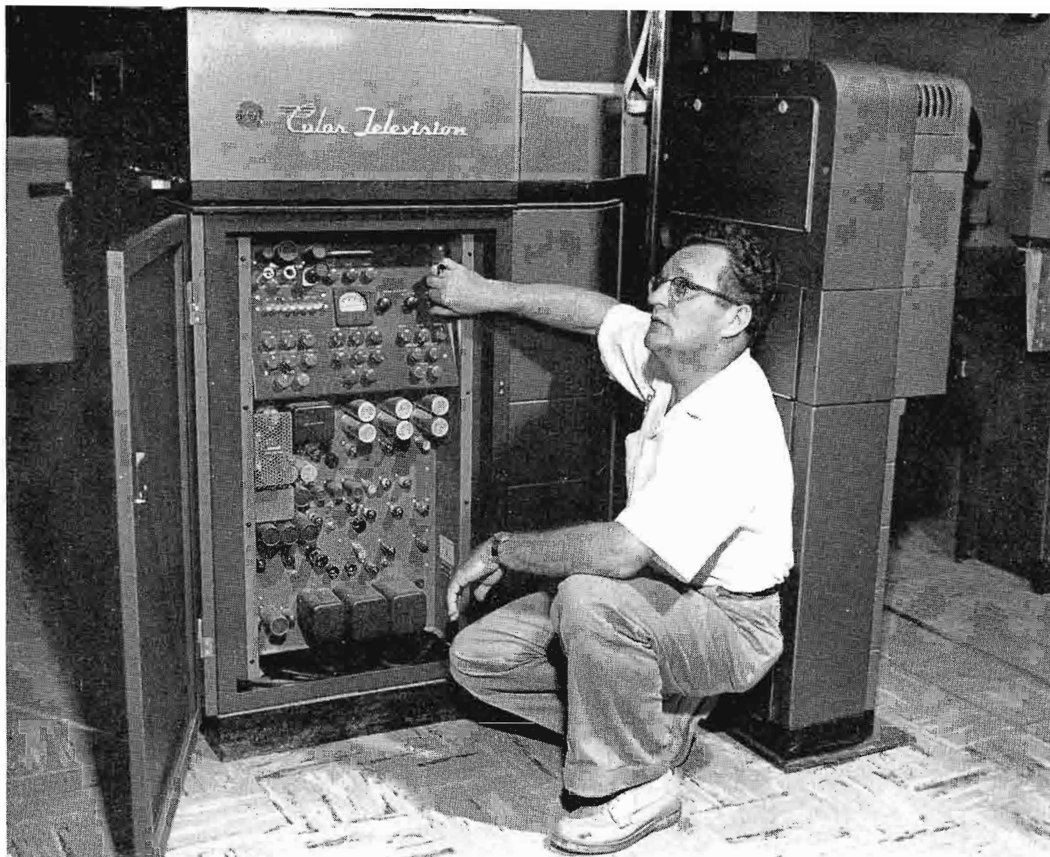
FIG. 16. RCA 3-V film system. Open door exposes control panel and camera auxiliary chassis . . . top cover houses optical system. RCA TP-6BC 16mm motion picture projector is shown at right.
