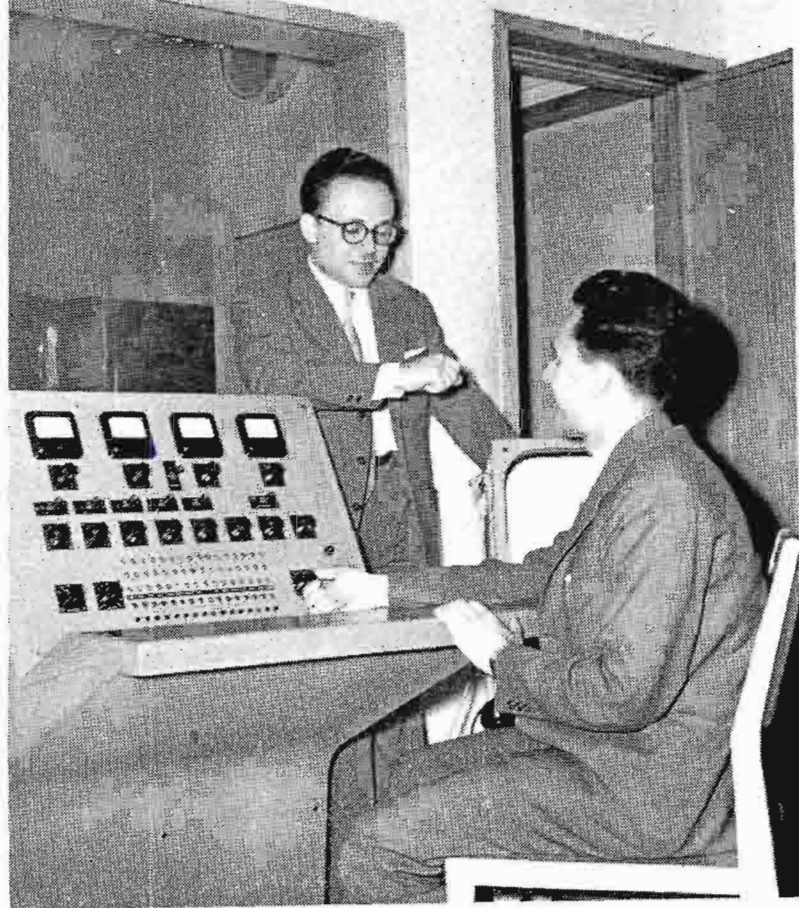
FIG. 15. Ing. Liverani and Marchese at audio switcher designed and built by the RAI engineers.
