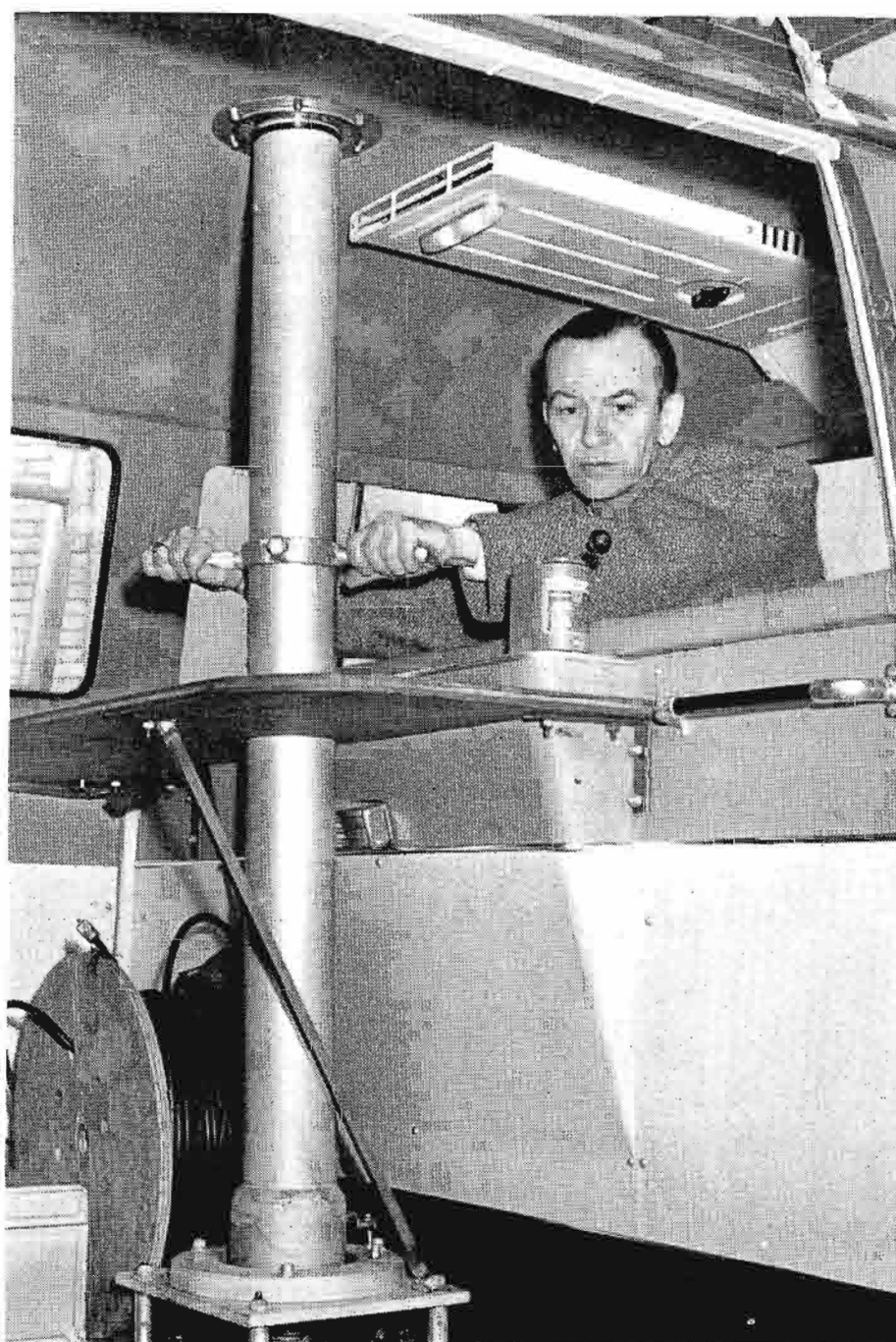
FIG. 2. View of hydraulic antenna mast control lever and facility for rotating.
