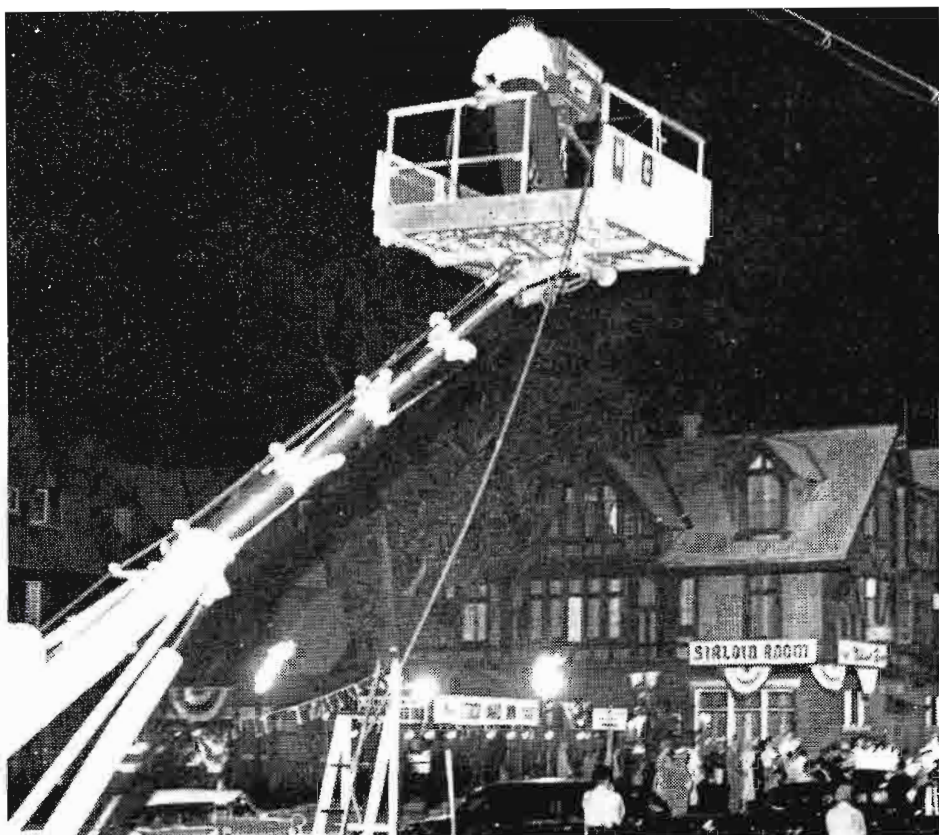
FIG. 1. TV camera operated from a Hi-Lift truck-mounted platform, capable of extending to a height of 70 ft was one of the devices used for obtaining difficult pickups. Here it is shown covering Adlai Stevenson's movement from the Stockyard Inn (shown above) to the Amphitheatre. Later on it saved the day on the occasion of the President's arrival at the St. Francis Hotel in San Francisco. With less than two hours to go after being unable to find a satisfactory outside camera location for this event, the Hi-Lift was set up at the hotel, cable connected with the NBC mobile unit and a picture fed to TV control—all in about one hour.
