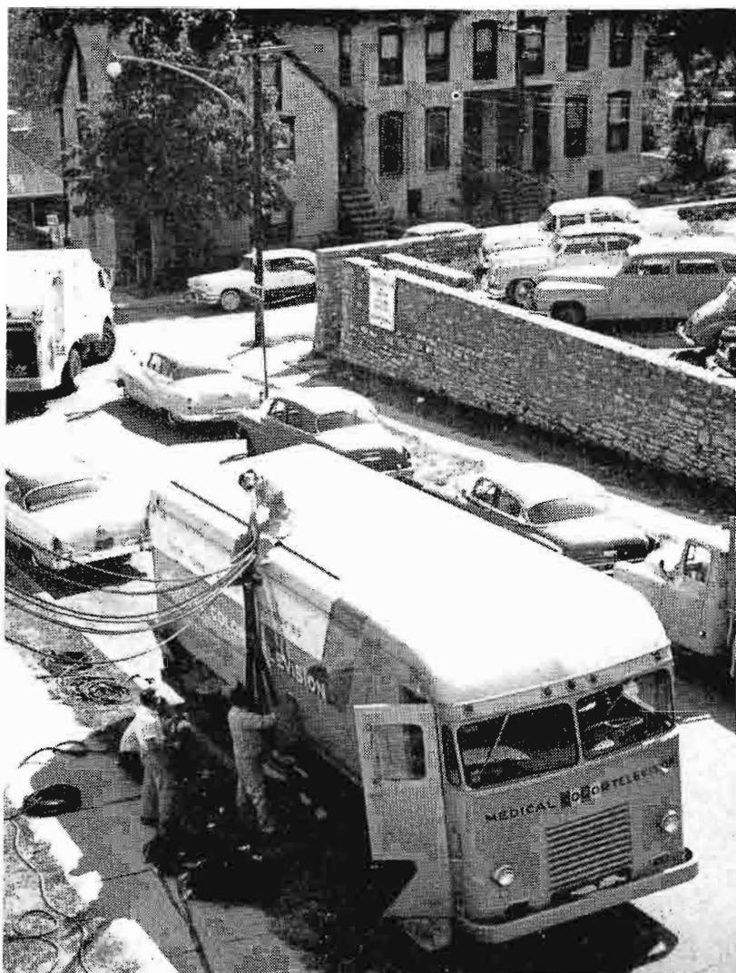
FIG. 13. Mobile unit is parked alongside hospital and connected to studio and power supply via cabling carried in the truck.
