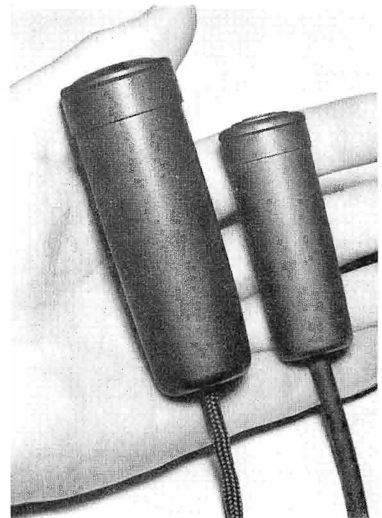
FIG. 5. A considerable reduction in size has been achieved in the BK-6B microphone (right) when compared to the BK-6A.
