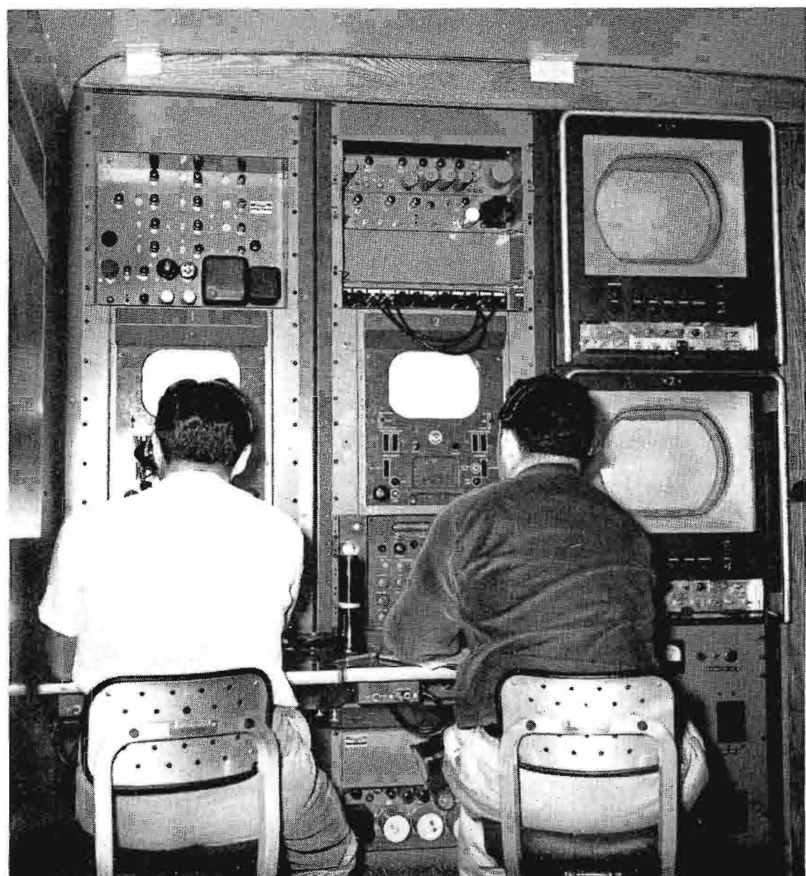
FIG. 17. When a TV demonstration is in progress, two technicians operate camera controls in mobile unit. Not seen is the technical director who operates switching.
