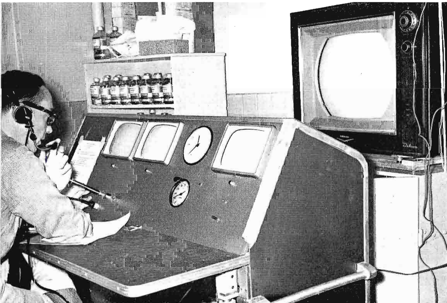
FIG. 19. Portable director's console, on wheels, contains miniature monitors fashioned from RCA 8-inch personal TV sets. Color receiver in background is used for live monitor.
