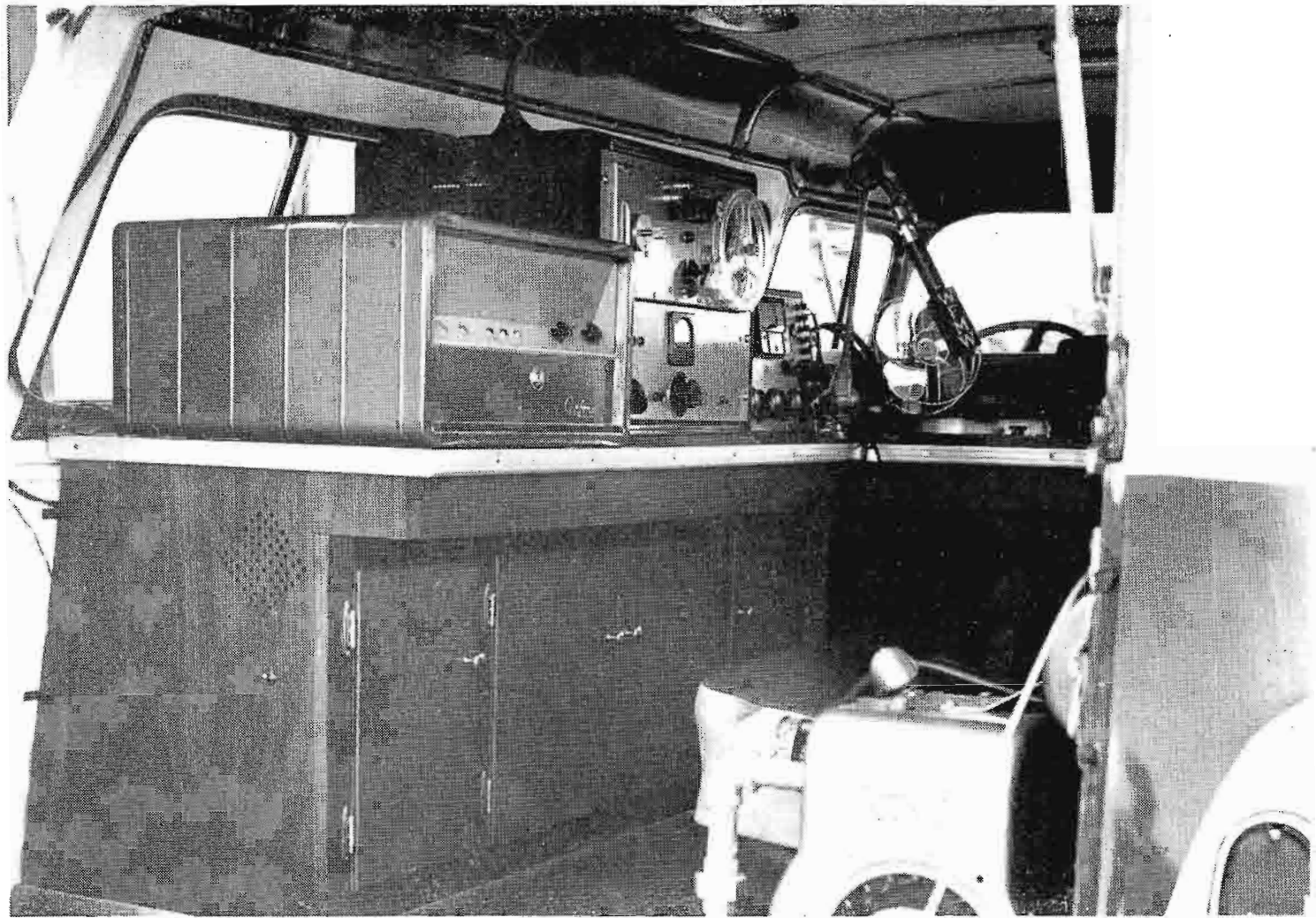
FIG. 4. This 500-watt gasoline generator mounted at the right rear of the mobile truck supplies enough power to operate all of the unit's equipment.
